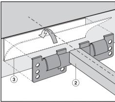
■ Position and attach the spring clips
